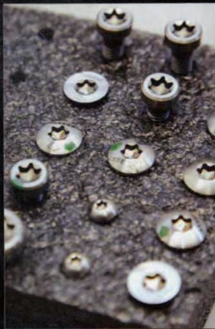
Top: Horacio talks aerodynamics. Right: rear view with flaps raised. Above: every bolt used on the car is titanium. Below: Xtrac gearbox is a transverse unit, offering better weight distribution
