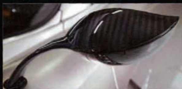
Above: new seats offer better support than Zonda's. Below: mirrors look delicate, but carbon construction makes them strong. Right: front flaps in raised position. Below right: wheels have a single central nut.
