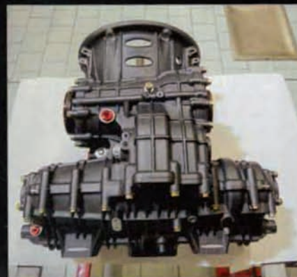
Top: Horacio talks aerodynamics. Right: rear view with flaps raised. Above: every bolt used on the car is titanium. Below: Xtrac gearbox is a transverse unit, offering better weight distribution
