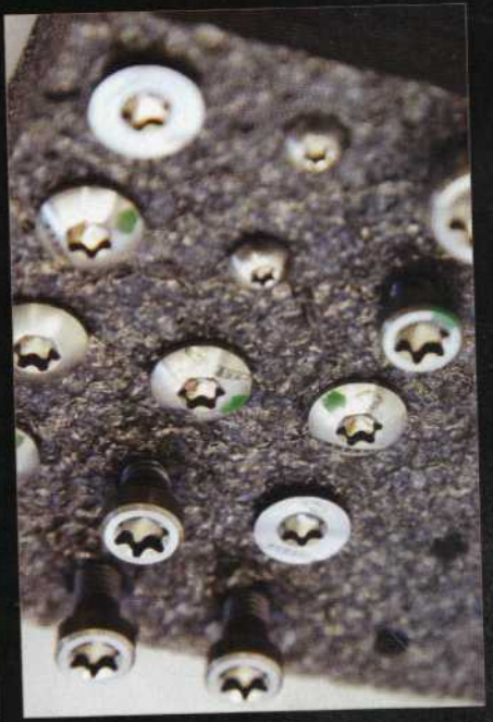
Top: Horacio talks aerodynamics. Right: rear view with flaps raised. Above: every bolt used on the car is titanium. Below: Xtrac gearbox is a transverse unit, offering better weight distribution
